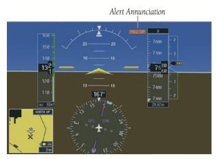
Figure 10-28 Alert Annunciation on the PFD
