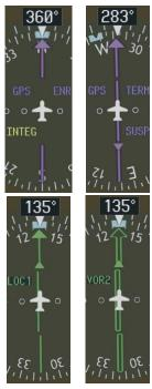
Figure 2-17 GPS INTEG, GPS SUSP, LOC1 and VOR2
