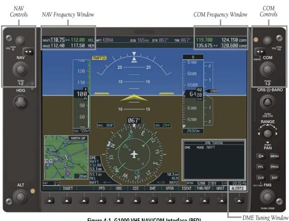
Figure 4-1 G1000 VHF NAV/COM Interface (PFD)
